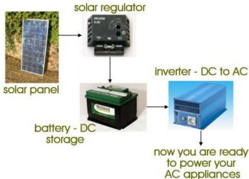
The **solar panel** converts sunlight into DC power or electricity to charge the **battery**. This DC electricity/(charge) is controlled via a **solar regulator** which ensures the battery is charged properly and not damaged and that power is not lost/(discharged). DC appliances can then be powered directly from the battery, but AC appliances need a **power inverter** to convert the DC electricity into 220 Volt AC power.
